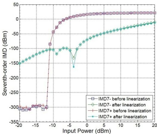
Fig. 9 Variation of 7<sup>th</sup>-order IMD with input power
