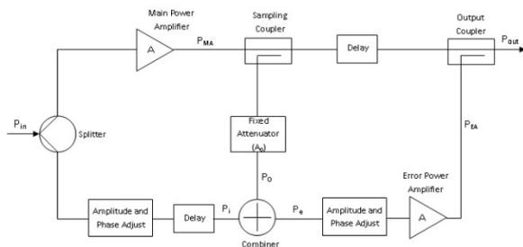
Fig. 2 Feedforward technique
