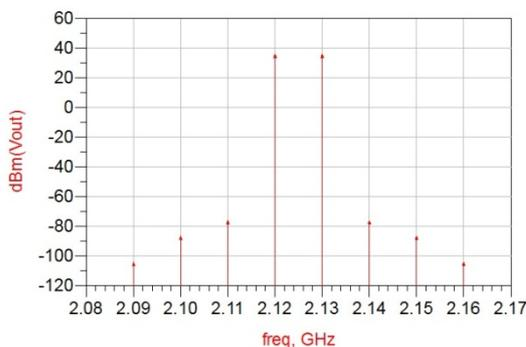
Fig. 6 Reduced IMD in amplifier output after linearization
