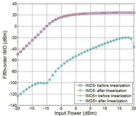
Fig. 8 Variation of 5<sup>th</sup>-order IMD with input power
