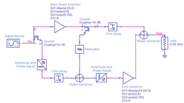
Fig. 3 Feedforward linearization circuit
