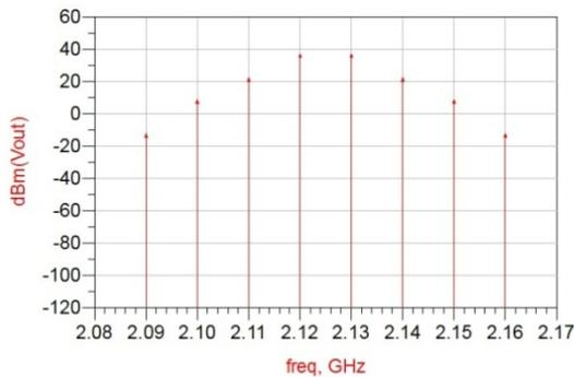
Fig. 5 IMD in amplifier output before linearization
