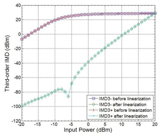
Fig. 7 Variation of 3<sup>rd</sup>-order IMD with input power
